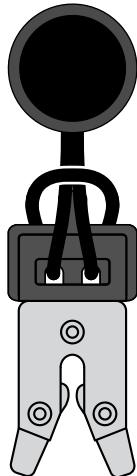
1) Taking one metal Alligator clip, rotate it so the smooth side is facing you, as shown in the diagram above.
